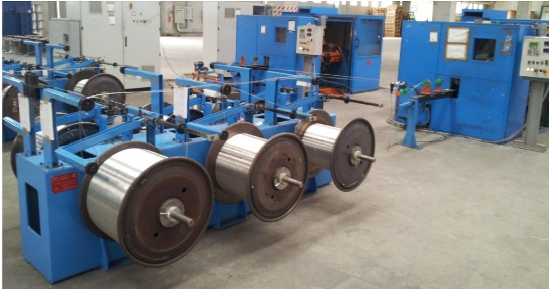
This double twist bunching machine is a highly productive machine used for the assembly of the following cables:
